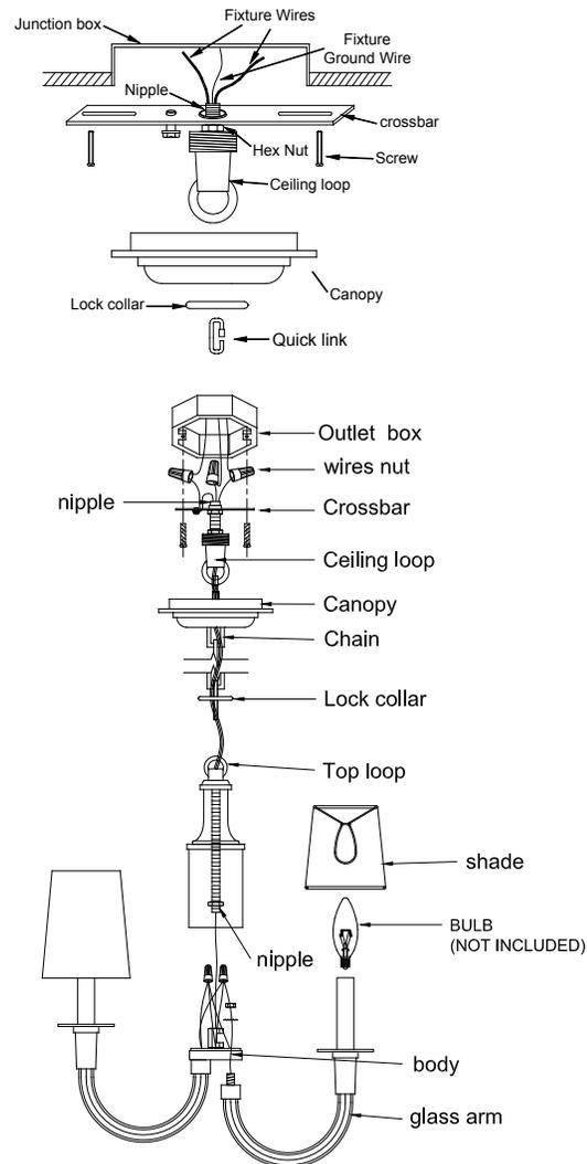
1. Install the ceiling loop into the top of the junction box. Leave the loop loose while you place the canopy and lock collar into place to set the depth of the loop. Once you have made certain that the canopy and lock collar will install easily, secure the ceiling loop, by tightening the hickey into place. Tighten all hex nuts using an adjustable wrench and a pair of pliers.
