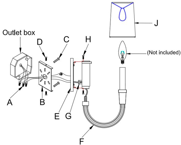
1. Remove plate (E) by unthreading screws (H) from the fixture.
