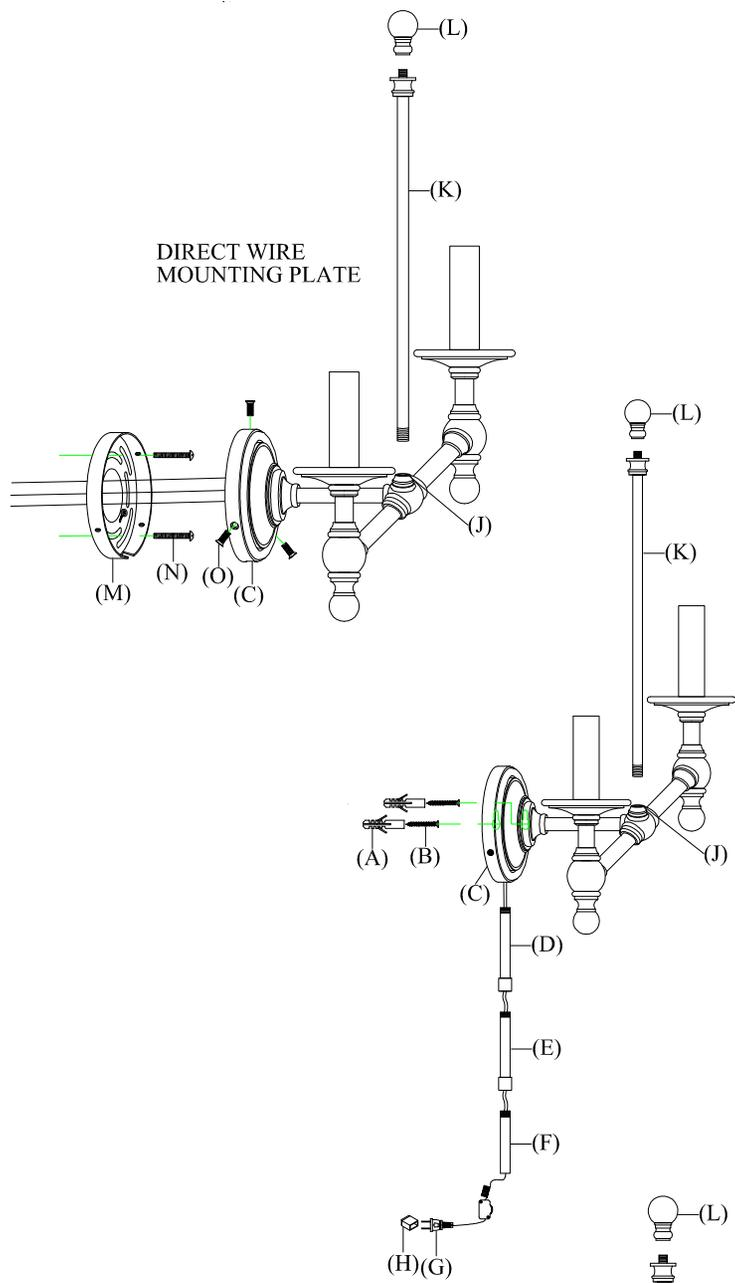
1. Screw threaded nipple of cord cover (D) into bottom threaded opening of back plate (C). Thread cord cover (E) into cord cover (D), thread cord cover (F) to cord cover (E) and hand tighten.
