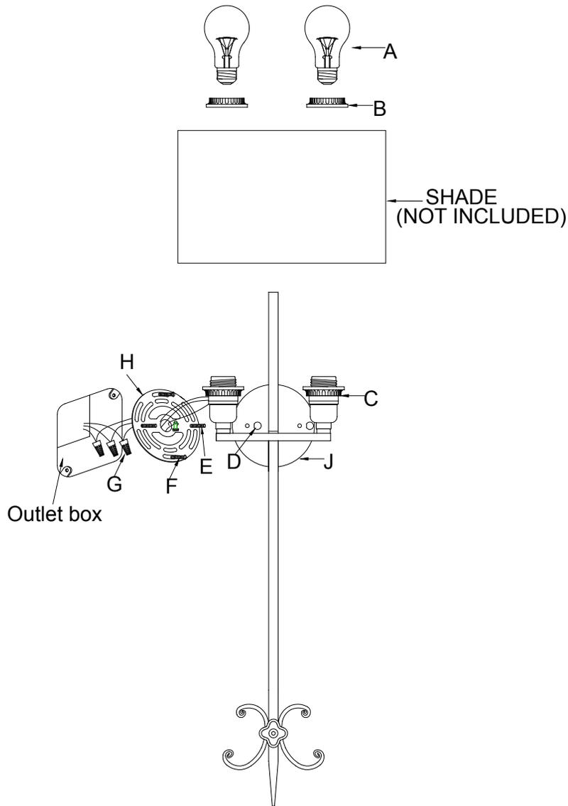
1. Carefully remove the mounting plate(H) from the back plate(J) by removing the two ball nuts(D).
