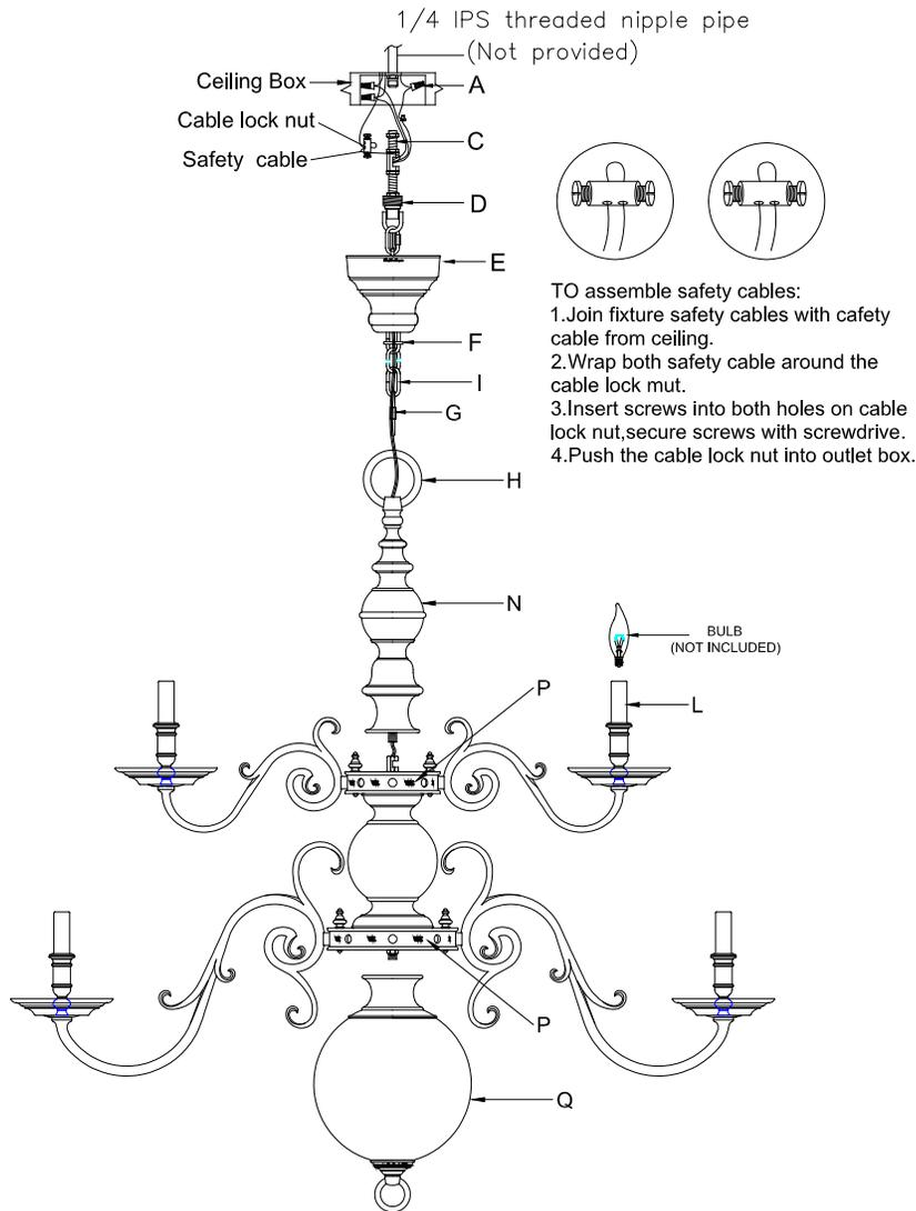
1. Install the threaded nipple (C) with hickey and nut into the ceiling box. You must provide a 1/4 IPS threaded nipple which will go through the top of ceiling box and through a structural member of building.
