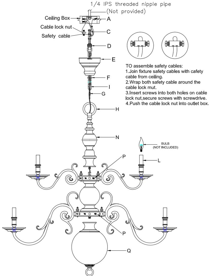
12. Connect the Ground (bare) fixture wire with the ground (usually bare) wire from your ceiling box using wire nut (A). If your house does not have ground wire, then attach this wire to the green grounding screw inside of outlet box. IT IS IMPERATIVE THAT THIS FIXTURE BE GROUNDED.
