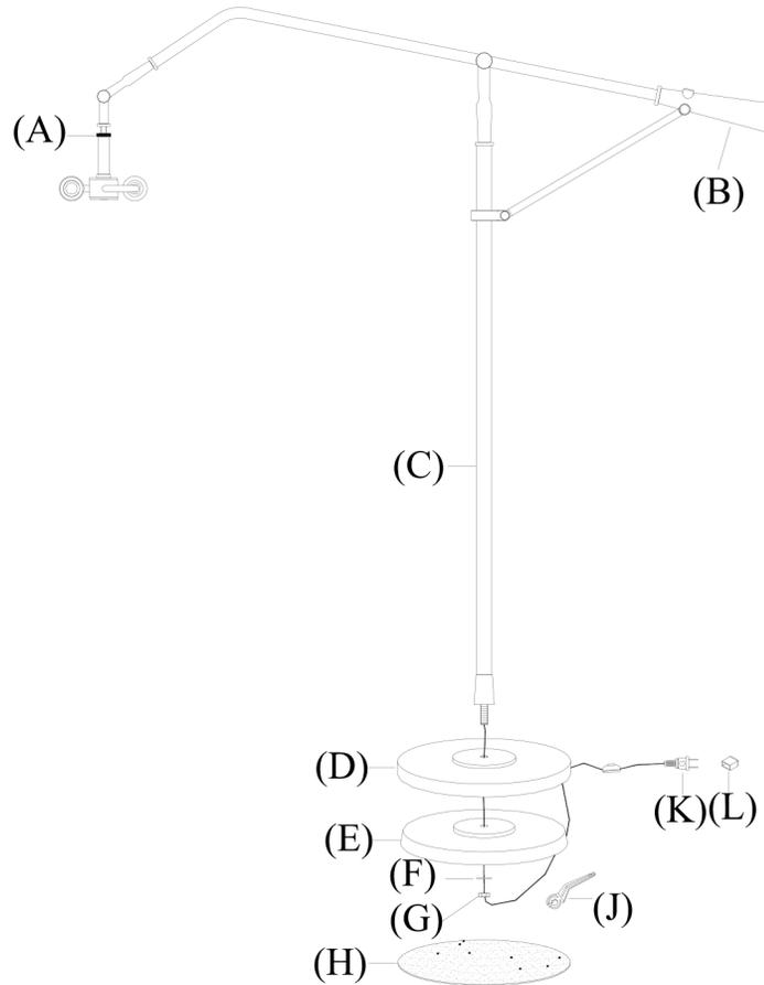
1. Join lamp pole (C), lamp base (D) and base weight (E) together by tightening washer (F) and nut (G) to threaded rod at bottom of pole (C). Tighten with wrench (J) provided.
