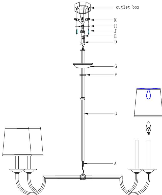
1. Insert the threaded pipe(A) with a nut on bottom into the fixture assembly(B) and tighten.
