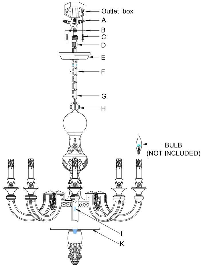
14. Connect the Ground (bare) fixture wire with the ground (usually bare) wire from your ceiling box using wire nut (A). If your house does not have ground wire, then attach this wire to the green grounding screw inside of outlet box. IT IS IMPERATIVE THAT THE J-BOX IN YOUR HOME BE PROPERLY GROUNDED.
