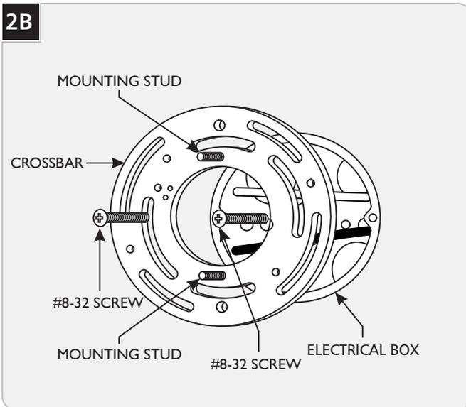
**2** Align the two mounting studs vertically and mount the crossbar to the electrical box with the two #8-32 screws provided.
