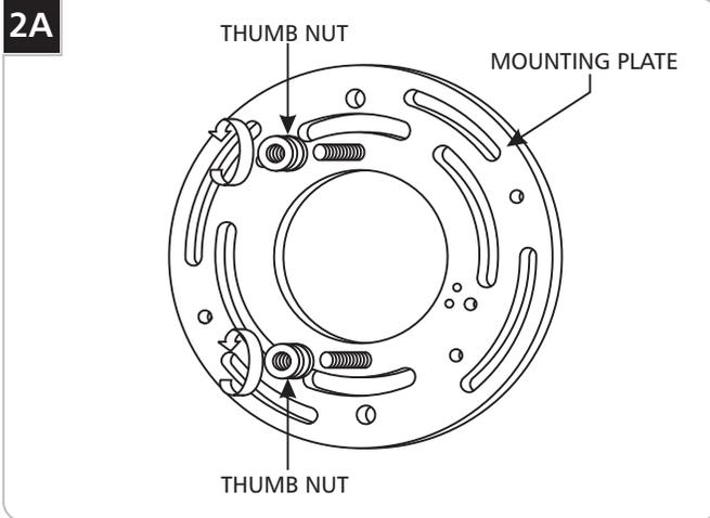
**1** Unscrew and remove the two thumb nuts from the mounting plate.
