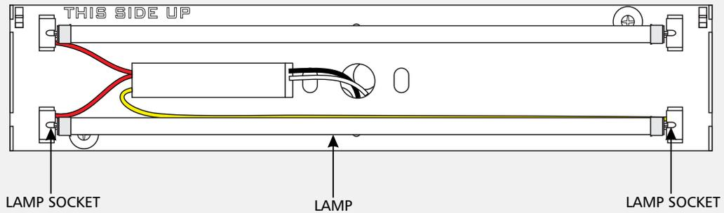
**CAUTION:** To reduce the risk of a burn or electric shock during relamping, disconnect the power to the fixture.
