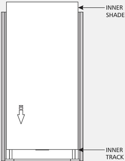
2 Gently slide the edges of the inner shade down the tracks in the fixture base until it rests against the end of the inner tracks.
