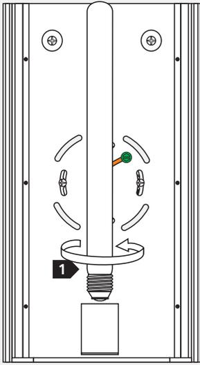
**CAUTION:** To reduce the risk of a burn or electric shock during relamping, disconnect the power to the fixture.
