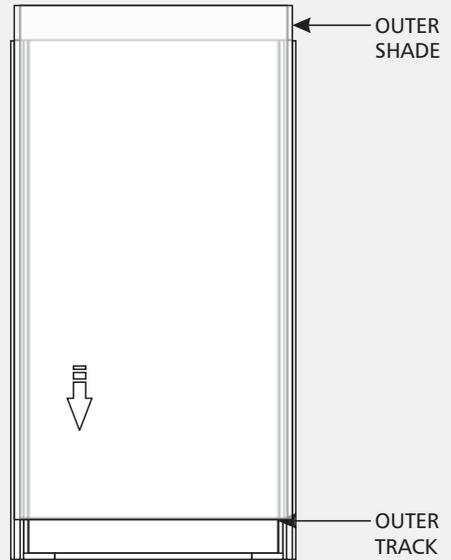
3 Gently slide the edges of the outer shade down the outer tracks in the fixture base until it rests against the end of the tracks.
