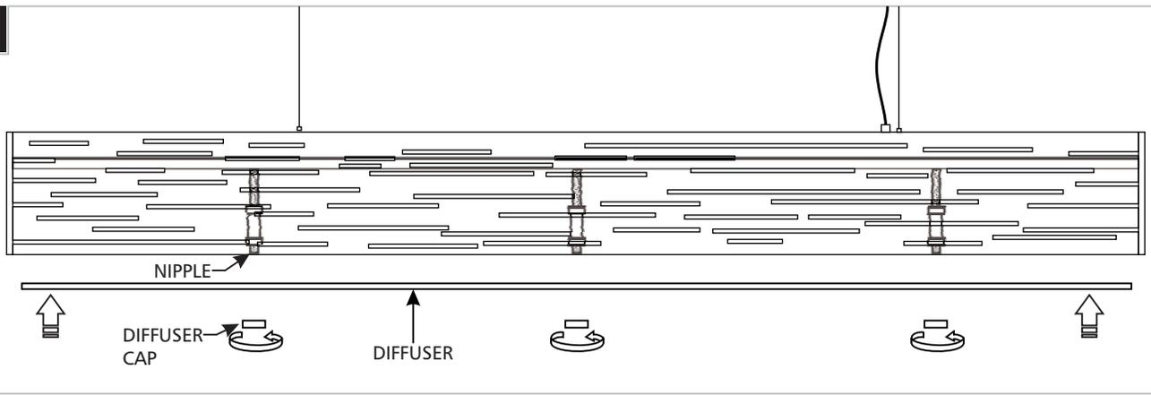
1 Place the diffuser onto the 3 nipples and secure it by completely screwing in the three diffuser caps.
