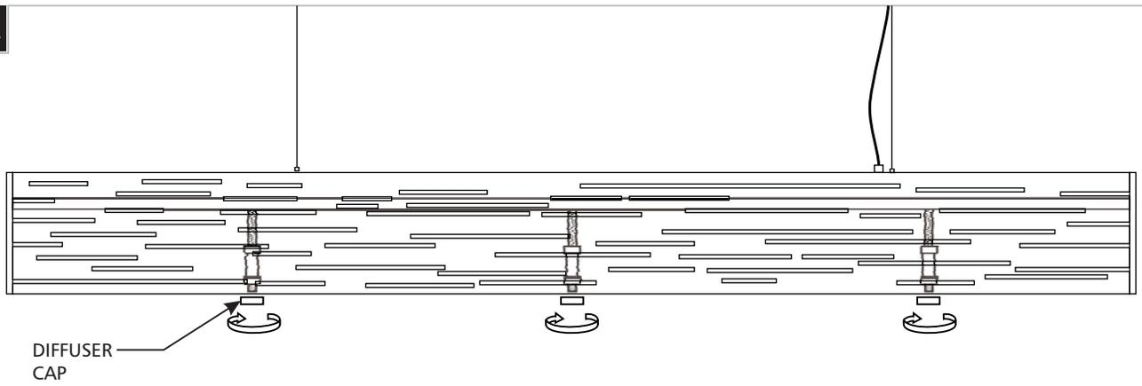
1 Loosen and remove all three diffuser caps.
