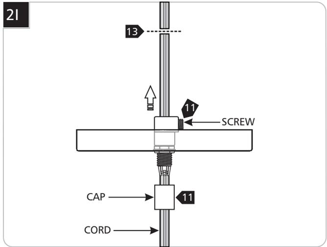
**NOTE:** The power cord does not support the fixture. For a casual "lazy cord" look, cut the power cord several inches longer than the drop height of the fixture.
