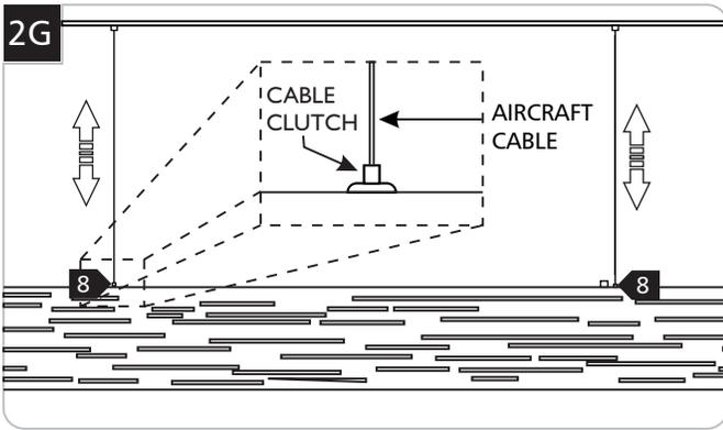
**8** Adjust the aircraft cables until the fixture is at the desired height and level; feed the cable into the cable clutch to raise the fixture and push in on the cable clutch nipple to release the cable and lower the fixture.
