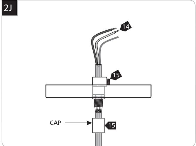
**14** Strip the cable behind the canopy, and strip the ends of the inner wires.
