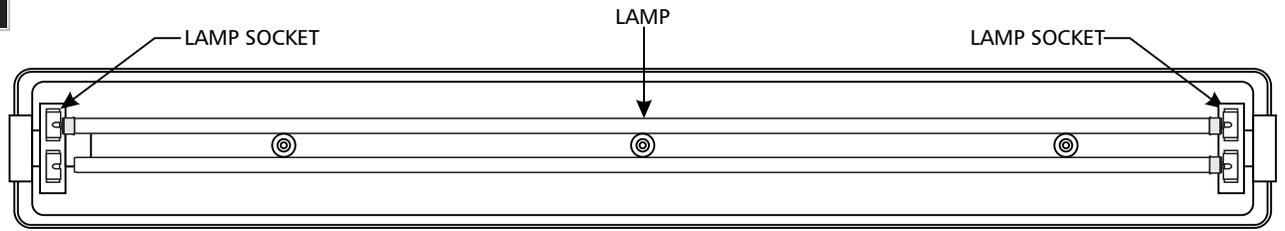
2 Line up the lamp pins into the sockets and rotate the lamps to lock it in place.
