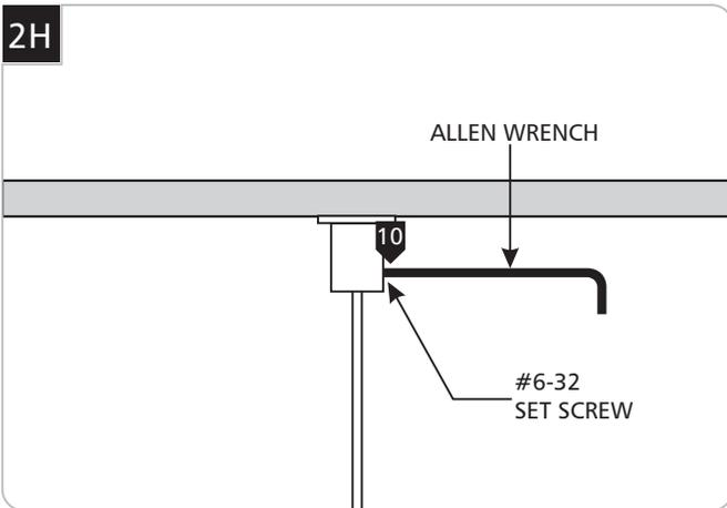
**10** Ensure that the set screws in both the canopy and the cable post are tight with the provided Allen wrench.
