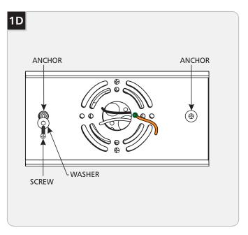
Slide a #8 screw through a washer, and screw it into an anchor to secure the fixture base to the wall. Repeat for the other anchor.
