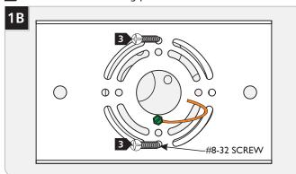
Install the mounting plate onto the electrical box with the two #8-32 screws provided.
